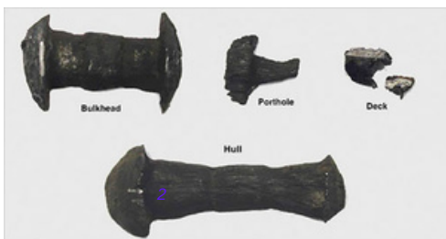
Figure 4 Rivets Recovered from the Wreck of Titanic
