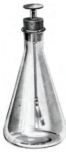
Figure 20. Another simple idea, an Erlenmeyer flask turned into an electroscope (Philip Harris Chemical and Physical apparatus Catalogue 1960)
