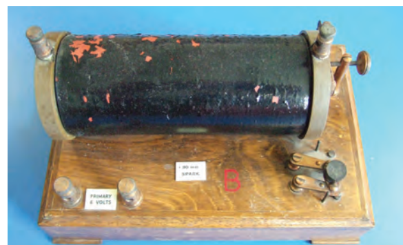
Figure 1. Philip Harris induction coil to generate high voltages (picture courtesy of Alex Marsh)
