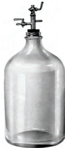
Figure 19. Clement and Desormes' Apparatus. By measuring air at two different pressures with a manometer, this simple glass bottle can be used to calculate the ratio of the two specific heats (Philip Harris Chemical and Physical apparatus Catalogue 1960)
