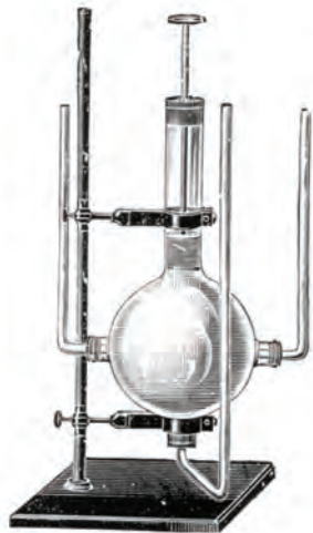
Figure 18. An apparatus to demonstrate the transmission of fluid pressure (Philip Harris Chemical and Physical apparatus Catalogue 1960)
