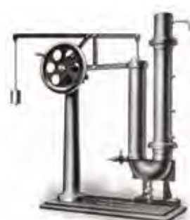
Figure 16. Apparatus based on the work of R. A. Henry for determining the washability of coal (courtesy of Ted Cook)
