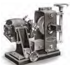
Figure 15. An apparatus for measuring the wear resistance of rubber by checking the weight of a sample after a number of rotations against an abrasive wheel. It was particularly aimed at tyre manufacturers (courtesy of Ted Cook)
