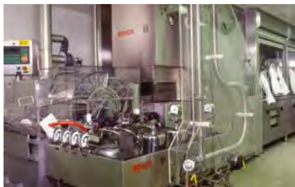
Figure 2 Isolator protected ampoule filling machine (Copyright: Cilag AG, CH-8201 Schaffhausen, image courtesy of Schicht Hans H.: 40 years of cleanroom technology - some historical remarks. In: Proceedings of the 17th International Symposium on Contamination Control, Bonn/Germany, 6-9 Sept. 2004, p. 1-10. Edited by: Verein Deutscher Ingenieure (Association of German Engineers), Düsseldorf/Germany (2004))
