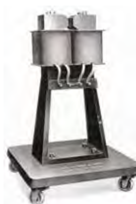
Figure 14. A hefty piece of kit. Three hundred kg of iron and 100 kg of copper wire went into the construction of this electromagnet, giving a magnetic field of two tesla (courtesy of Ted Cook)
