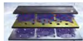
Fig. 2: Graphene electrochemical capacitor. Two high-surface-area graphene-based electrodes (blue and purple hexagonal planes) are separated by a membrane (yellow). Also shown are anions (white and blue merged spheres) and cations (red spheres) of the electrolyte (Source: reference 4 )
