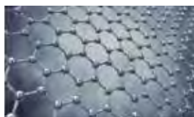
Fig. 1: Graphene - monolayer of carbon atoms packed into a dense honeycomb crystal structure. This is viewed as an individual atomic plane extracted from graphite (Source: Wikipedia image)
