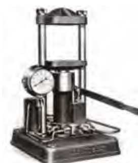
Figure 13. The Cook laboratory hydraulic press, available in various versions up to 50 tons pressure (courtesy of Ted Cook)
