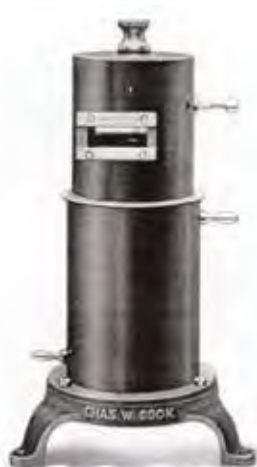
Figure 1. Looking a little like a paraffin stove, a gold leaf electroscope said to have been designed by Ernest Rutherford (courtesy of Ted Cook)
