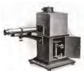
Figure 2. A combined alpha-beta-gamma electroscope described as Dr Lazarus-Barlow type (courtesy of Ted Cook)
