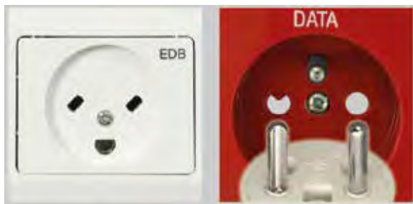
Left: Danish EDB socket with slots for angled flat pins, rather than standard round pins. Right: Polish data socket and plug; the left pin has a V-shaped groove. EDB and DATA devices are used for powering electronic equipment.
