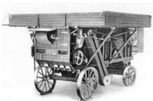
Figure 4. A model of a threshing machine made from oak and polished aluminium, about one quarter scale. It appears in the c.1953 catalogue but was made at Manchester prior to 1912
