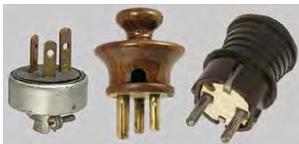
Examples of classic earthed pins. Models are still in use. Left: Hubbell plug, designed by George Knapp (from 1938 Australasian standard plug). Middle: wooden Tripin-like 5A plug (comparable to BS 546). Right: early 1930s Schuko plug with earth clips (essentially unchanged in almost 90 years).
