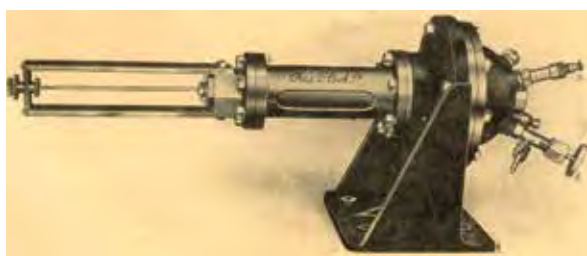
Figure 19. A spherical chamber for the combustion or explosion of gases. It is fitted with a pressure gauge devised by Joseph Petavel. Shown in the 1955 Chas W. Cook & Sons Ltd catalogue (courtesy of Professor Hans Michels)
