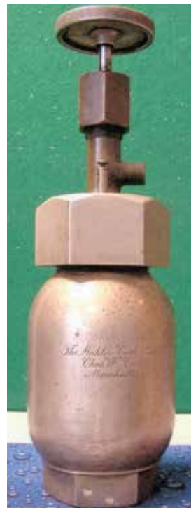
Figure 3. The inner part of a Mahler-Cook bomb calorimeter made at Manchester. It was used as a doorstop in more recent times (calorimeter saved for posterity by Mike Allsop)
