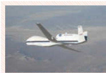
NASA's Global Hawk, a remote-controlled airplane that can fly for up to 30 hours at altitudes up to 65,000 feet.
