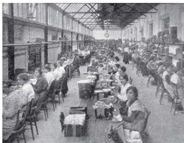
Gas mantle manufacture: Sewing gas mantles at the Volker Lighting Corporation (Tilden)
