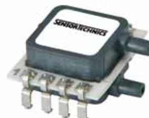
Figure 7 A precision compensated pressure sensor from Sensortech.
