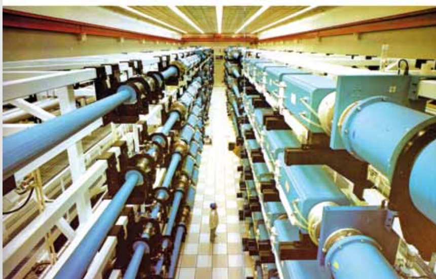
Lasers range in size from microscopic diode lasers (top) with numerous applications, to football field sized neodymium glass lasers (bottom) used for inertial confinement fusion, nuclear weapons research and other high energy density physics experiments.
