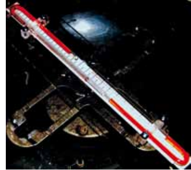
Figure 12 A strobe photograph of a Centrifugal Absolute Barometer while rotating.
