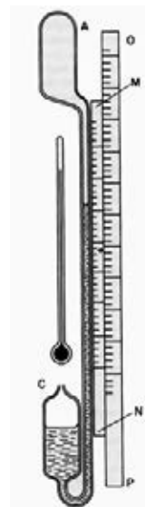
Figure 2 Adie's Sympiesometer. Sketch from Adie's Patent of 1818.
