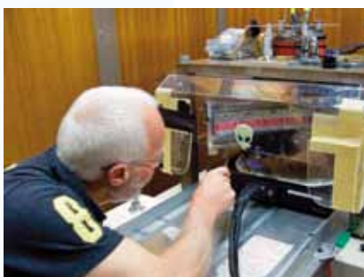
Aligning optical fibres on the imaging plate for the UK Schmidt Telescope.
