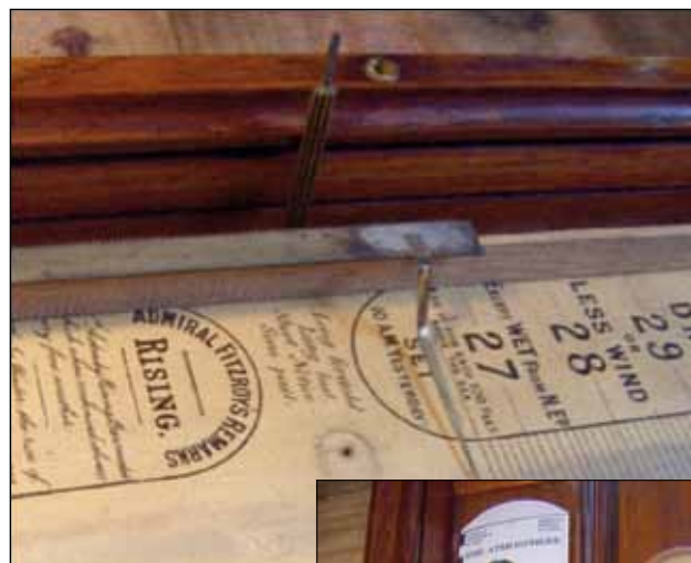
Figure 3. The Rack and Pinion index mechanism
