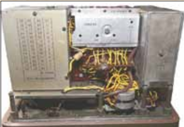
Figure 10 — Chassis — underside, showing screening plate.
