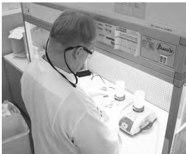
Figure 1: Work being undertaken in a laminar airflow cabinet (photograph courtesy of Bio Products Laboratory)
