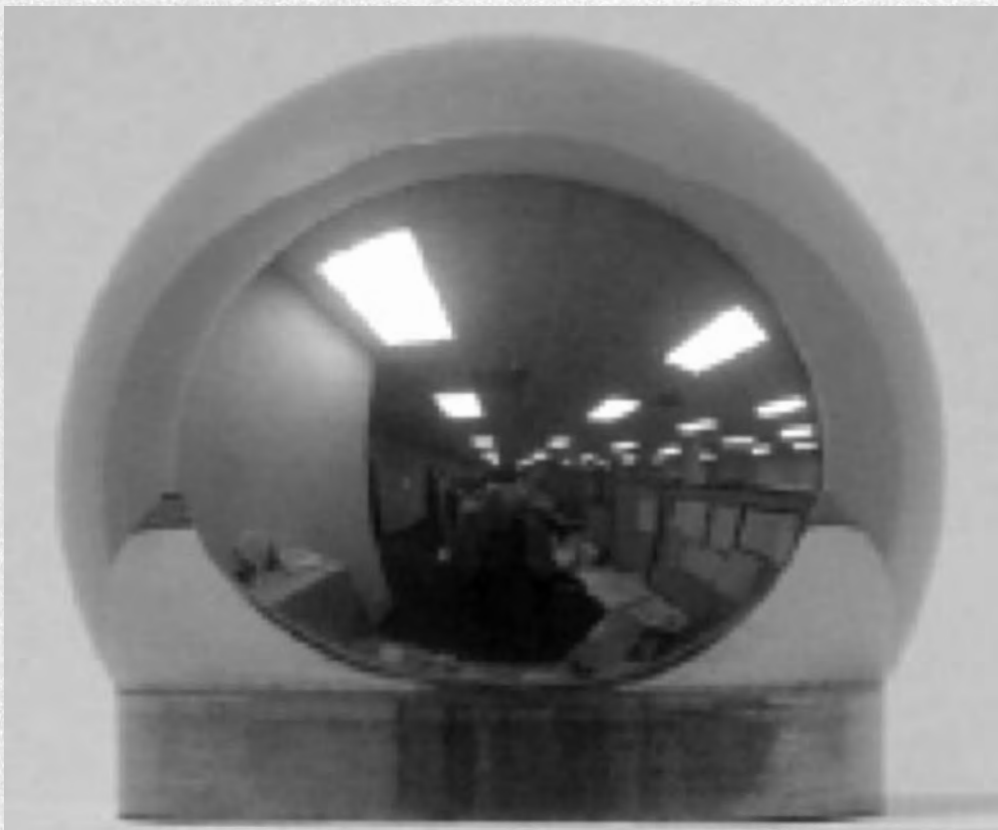
Blow moulded metallic glass at 460°C
